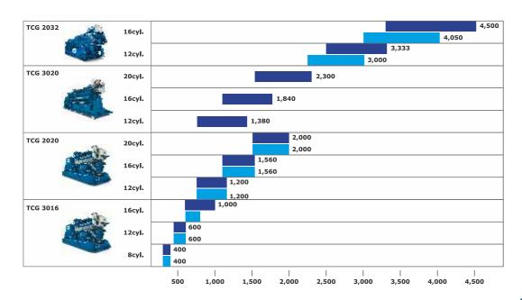
With our gensets, we can cover a power range from 400 kW to 10300 kW for decentralized power production.
